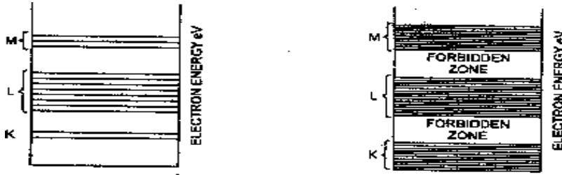
Figure -3.3 (b) Energy band representation of ionisation
